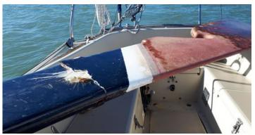
Above is the photo of the rudder of the Contessa removed from the stern of the boat and sitting in the cockpit for inspection. A large transverse crack was evident. This rudder was very close to breaking completely into two parts. Below shows the bracket in place ready to be glassed in and make the rudder strong for many seasons yet.
